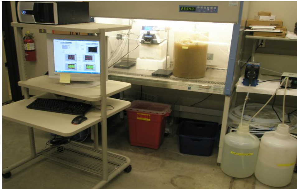
Figure C-2. Photograph of the designed bench-scale MBR system
