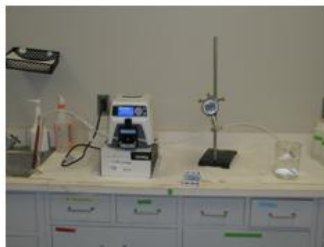
Figure C-1. Schematic and photograph of permeability test setup
